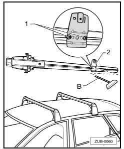
Insert the sliding blocks -1- of the bicycle carrier into the roof racks from the side, and adjust this to the desired position.
